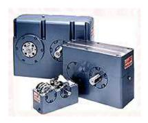
**IMC Parallel Index Drives** feature two plate cams mounted as a conjugate pair. The follower wheel has one cam follower above and another below the center line of the input, producing a preloaded locking action. Parallel indexers are capable of producing high speeds, large output displacements and low number of stops. Their input and output shaft design is best suited for any type of inline conveying system, shuttle drives and lift-and-carry mechanisms.
