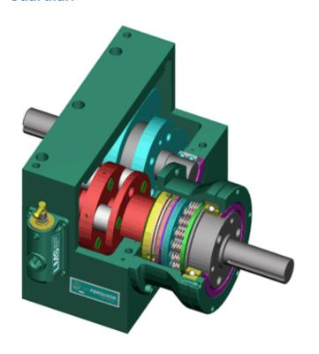
The Guardian Series parallel index drive includes all the features of the **Parallel series** along with an **Internal Torque Limiting Clutch**. The internal clutch provides design and assembly flexibility and reduces critical debugging time. Also ideal for harsh environments.
