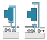
Parallel grippers can also be used for separating parts. A Gripper closing - all the balls are retained B Gripper opening - one ball is released, the others are retained.
